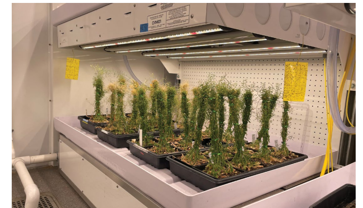
MTPS Flex growing Arabidopsis with optional far red spectrum LED lights.
