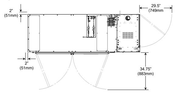
Figure 2-1 Installation Clearances
