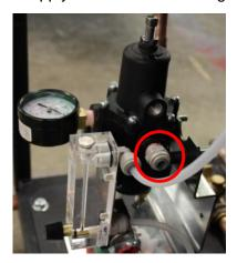
Figure 2-10 C0<sub>2</sub> Supply Line Connection
