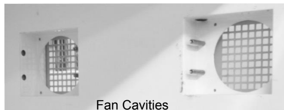
Figure 2-9 PG Fan and Air Inlet Cavities
