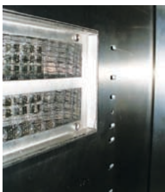
Figure 2.22: Canopy air inlet filter is showed.
