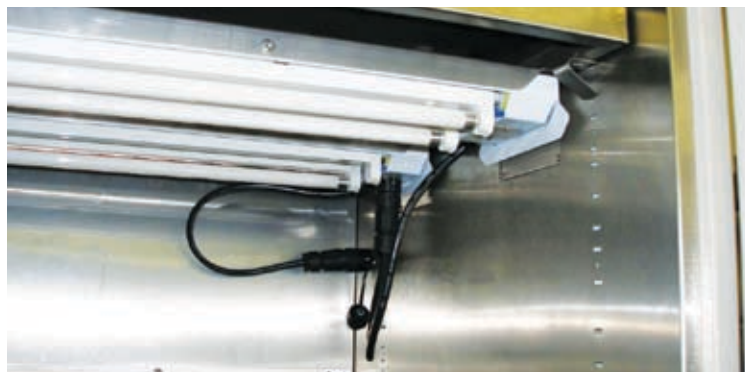
Figure 2.17: Lamp fixtures assembled and plugged.
