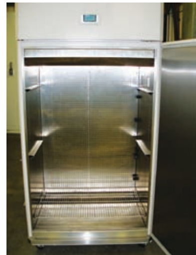
Figure 2.42: Canopy support showed with 18" (450 mm) between them for maximum growth height.
