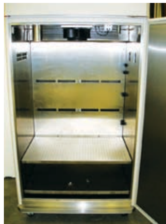
Figure 2.8: A1000 view after installing the first shelf.
