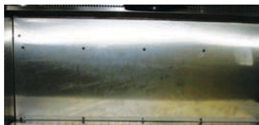
Figure 2.11: 5 screws installed at the back plenum before installing the top shelf.
