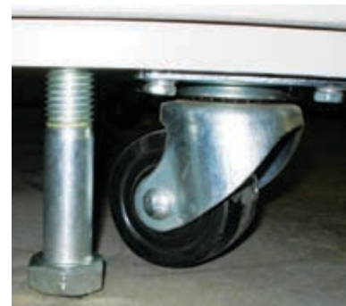
Figure 3.1: Unit raised with level bolt.
