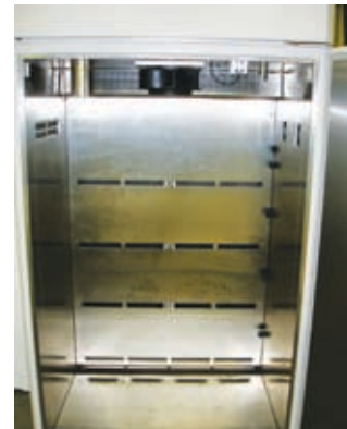
Figure 2.3: A1000 view after installing the back wall plenum.
