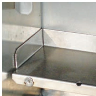
Figure 2.2: A1000 view after installing the back plenum bottom panel.
