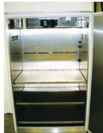
Figure 2.9: A1000 view after installing the second shelf.
