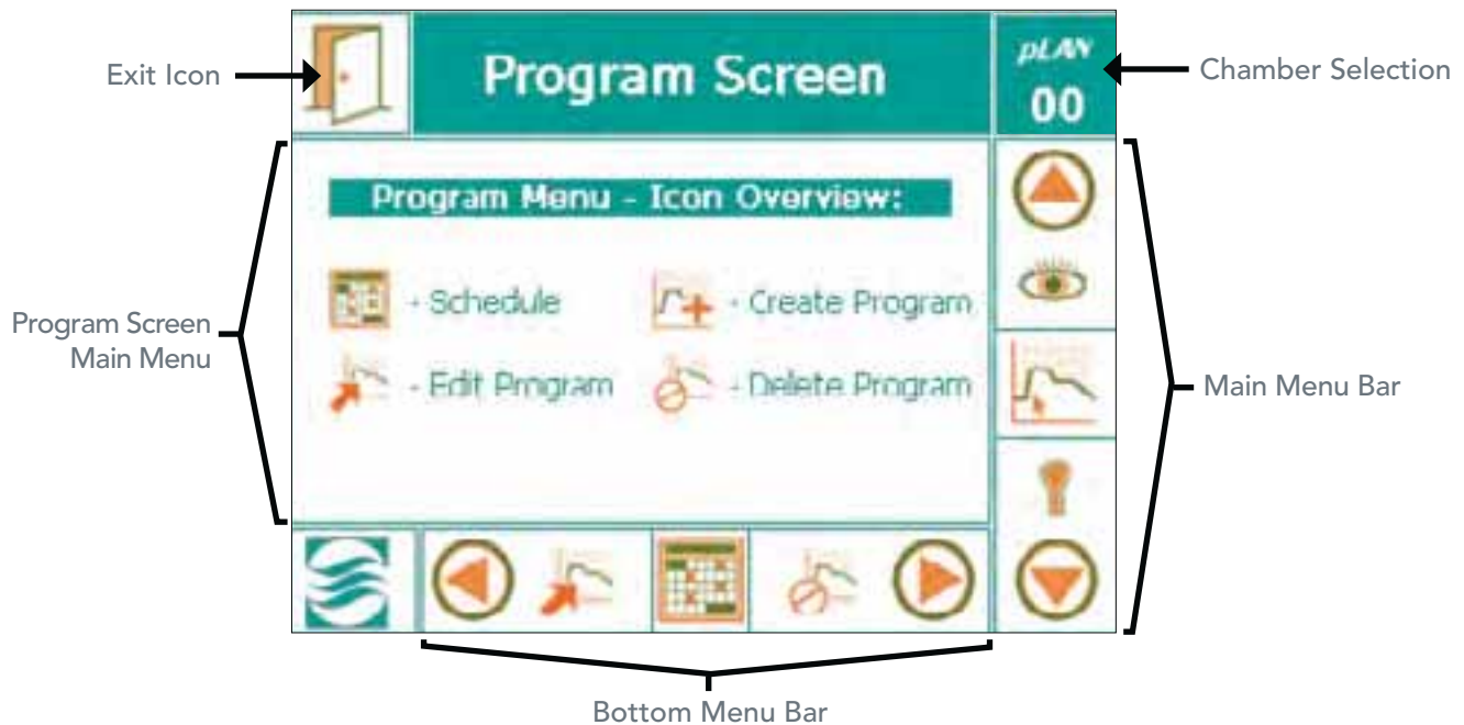
Figure 5-1: Program Screen – Key Area Layout
