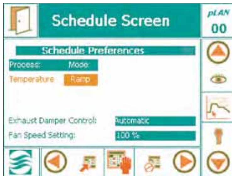
Figure 5-22: Fan Speed and CO 2 Exhaust Damper Setting
