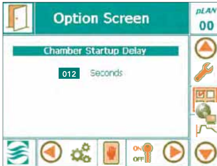
Figure 8-4: Chamber Start-up Delay
