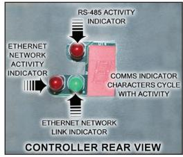
Figure 6.21: CMP5090 Indicator LEDs
