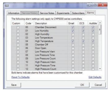
Figure 3.25: Chamber Alarm Settings
