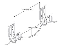
Figure 6.3: J-Hook Cable Supports
