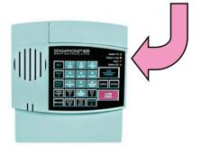
The Autodialer will respond to an alarm by dialing up to four separate telephone numbers. When the call is answered, an "Alert Condition" message is delivered and a userrecordable voice message. The Dial out sequence can be "acknowledged" by sending "555" from the phone keypad during a received call. This ceases dial out.
