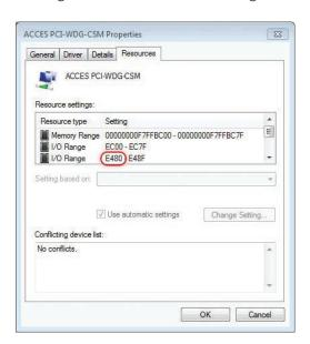
Figure 6.26a: Alarm Card Address
