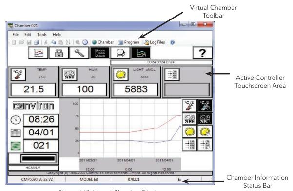
Figure 4.13: Virtual Chamber Display
