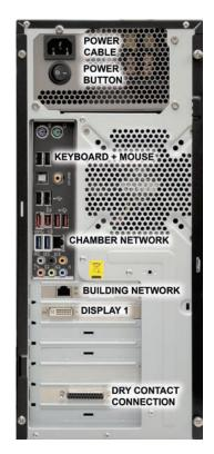
Figure 6.7: Central Management™ **PC** Connections
