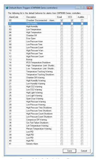
Figure 3.24: Default Alarm Triggers
