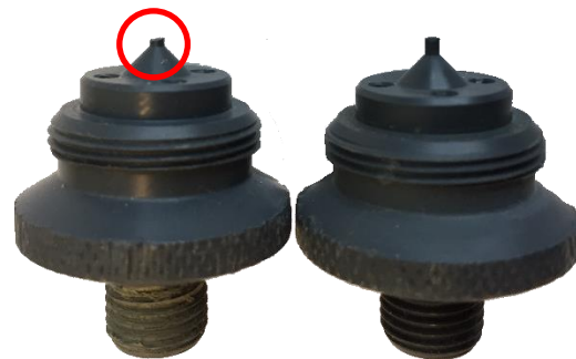
Figure 5-5 Damaged Orifice Tip
