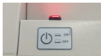
Figure 3.8: Main power switch
