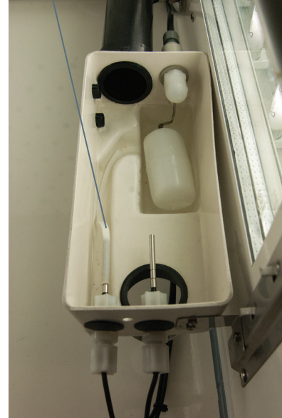
Figure 3.3: Aspirator interior showing wet wick
