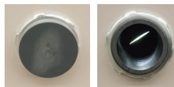
Figure 3.11: Instrument Port: Closed and Open
