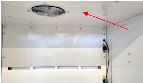
4. Re-install Ceiling Cover over TC Plenum.
