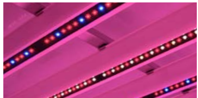
Nunhems utilizes mixed spectrum in the range of 400-700 nm; 50% deep red-white and 50% deep red-blue.
