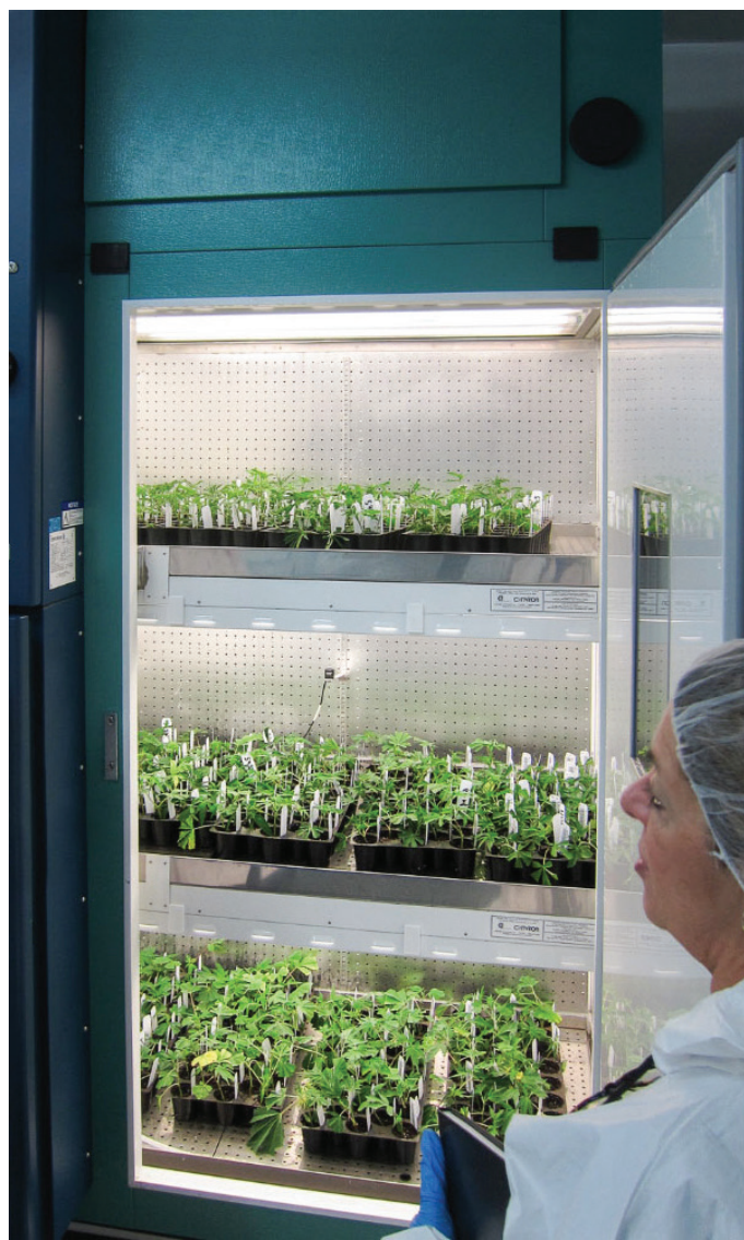
Reach-in plant growth chamber for cannabis clones
